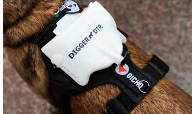
The SMART harness for mine detection dogs only weighs 700 grams, with its battery running up to 4 hours.
