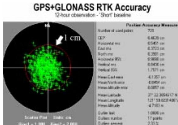
This plot was obtained from 12 hours of GG-RTK position data, with a short baseline. In this example the accuracy is well better than the specified accuracy. The horizontal rms accuracy of these RTK positions is 0.5cm. The worst case error is 1.3cm
