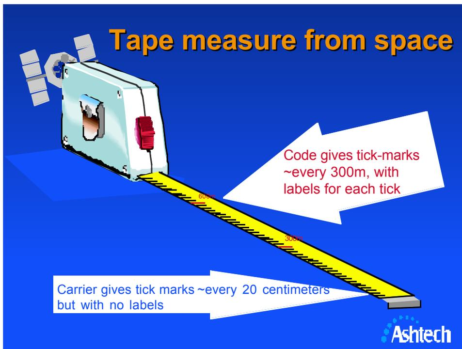
The GPS satellites provide the equivalent of a tape measure from space. The tape has labeled tick-marks at ~300m intervals (the code), as well as unlabelled tick-marks at ~20cm intervals (the carrier). A receiver can measure the code to 1m precision, and the carrier to one centimeter precision. A receiver that can compute the 'labels' on the carrier can then deliver centimeter position accuracy. This is what RTK receivers do.
