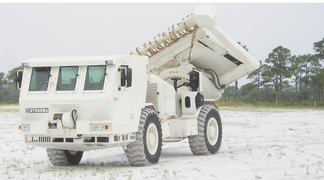
HYDREMA | Moving flail unit from transport to clearance position
