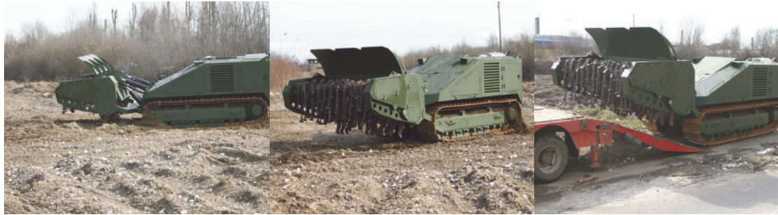
MV-10 | In service, detailed view of the working tool, driving on a flat bed trailer
