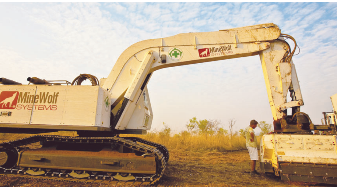
MINEWOLF BAGGER | With tiller attachment
