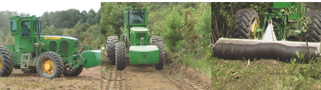
THE PEARSON MINEFIELD TRACTOR | Mine comb in heavy vegetation | Area reduction roller
