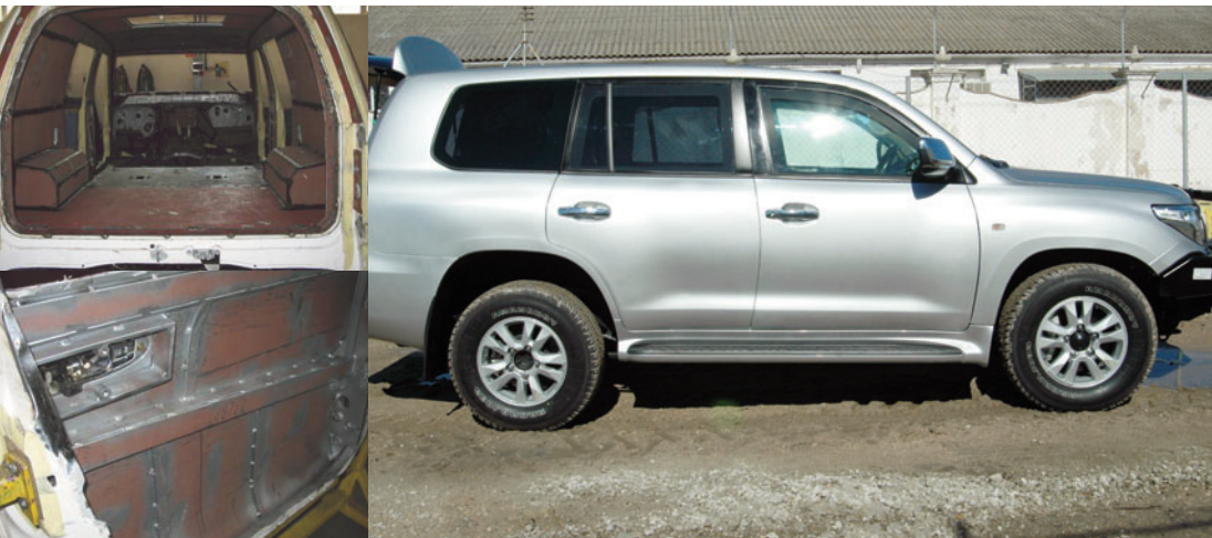
Putting in armour and finished exterior
