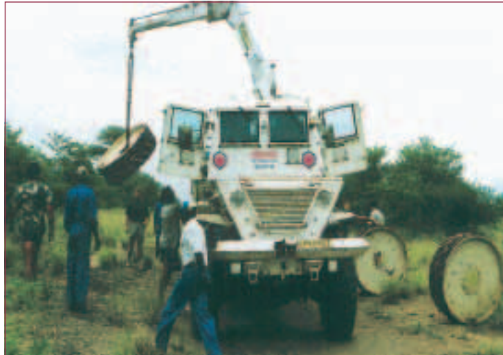
Early version of Casspir mounting steel wheels
