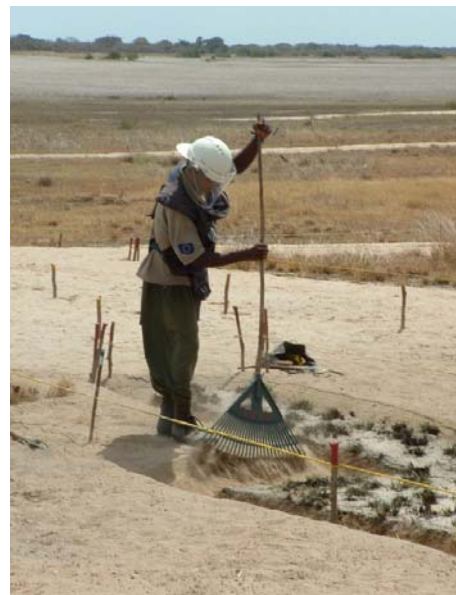
The picture above show the Brush-rake and Harrow-rake in use on HDU sites.
