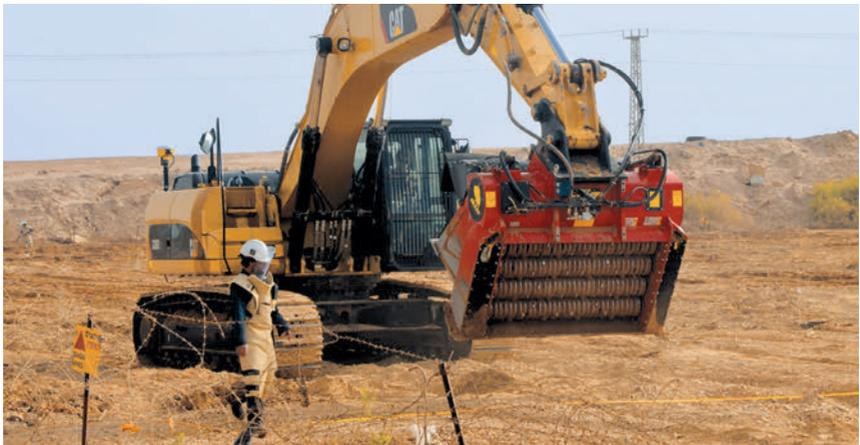
Mechanical crusher and sifter at work
