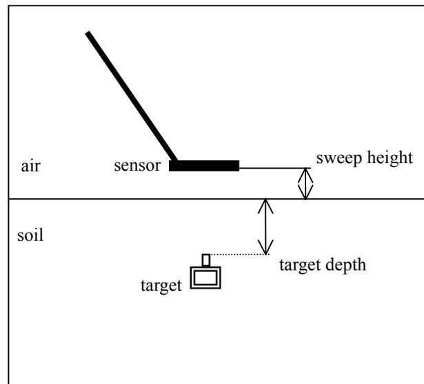
Figure 1 — Geometry for Testing Metal Detectors
