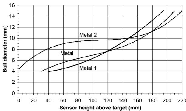
**Figure 2 — Minimum Target Detection Capability Curves for Balls of Three Metals**
