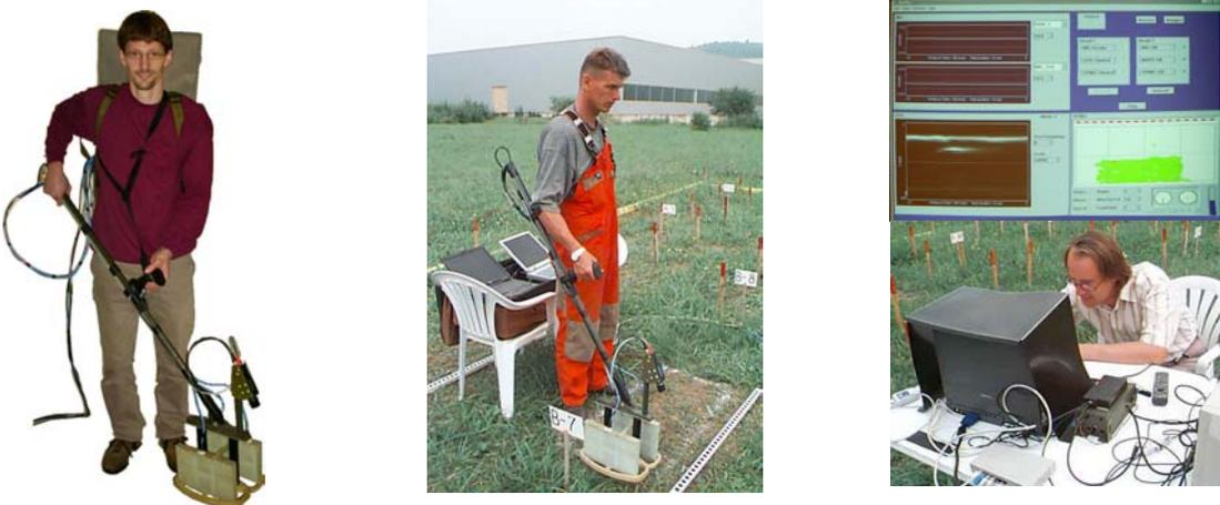
(a) The detector head and the backpack. (b) The detector head, the backpack (opened) and the marker bar. (c) The MMI notebook and the MMI screen.
