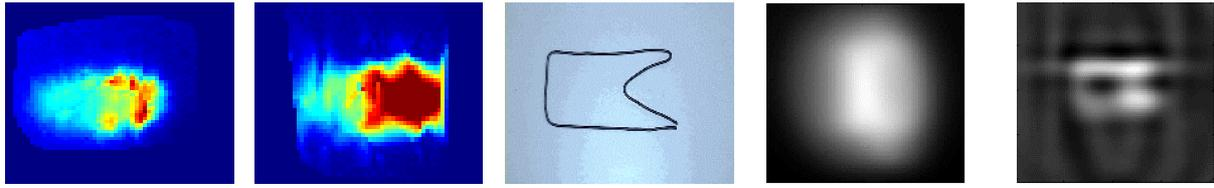
(a) Shallow metallic sphere      (a) Shallow barbed wire      (c) picture of the object      (d) raw MD image      (e) focused image
