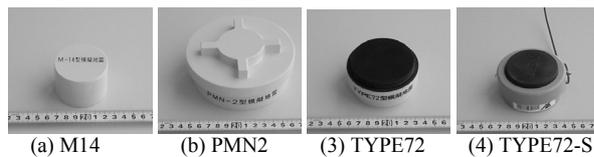
Fig. 5. Landmine surrogates used in test.
