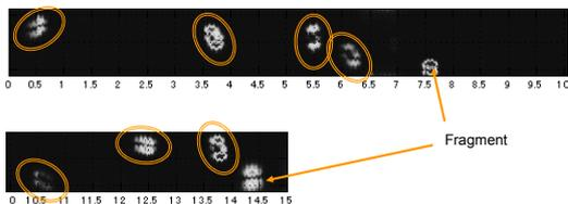
Fig. 11. Detection image from a metal detector.
