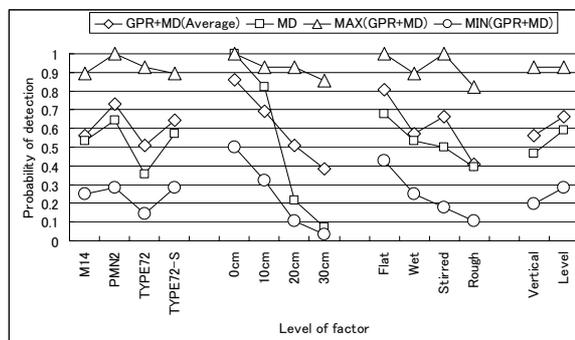
Fig. 13. Average PD for each level of factor of Experiment I.
