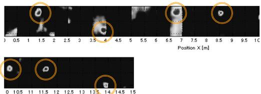
Fig. 12. Detection image from a GPR.
