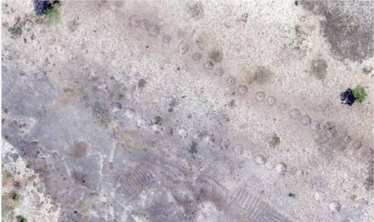
Figure 7. Craters from controlled demolition of anti-vehicle mines in a minefield in Cuito Cuanavale.
