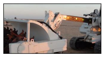
The Armtrac 400 has a Telescopic Boom to which different demining toolkits can be attached. This boom can be extended to clear mines and UXO in difficult locations such as on river banks and on inclines, while remaining completely stationary. This is a unique feature to the Armtrac tracked machines.
