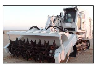
The Armtrac 400 is the largest and most powerful of the Armtrac range. With its hydraulically driven 3 meter Tiller rotor, it is capable of clearing 2,400 square meters per hour (depending on terrain & operator experience). With an effective tilling depth of 55cm the Armtrac 400 is designed to destroy & withstand 10kg Anti-Tank mines.
