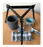
The Hot Drop system is astand-off method of melting a hole in an article of ordnance and burning the HE contents. The system consists of a crucible containing a charge of
