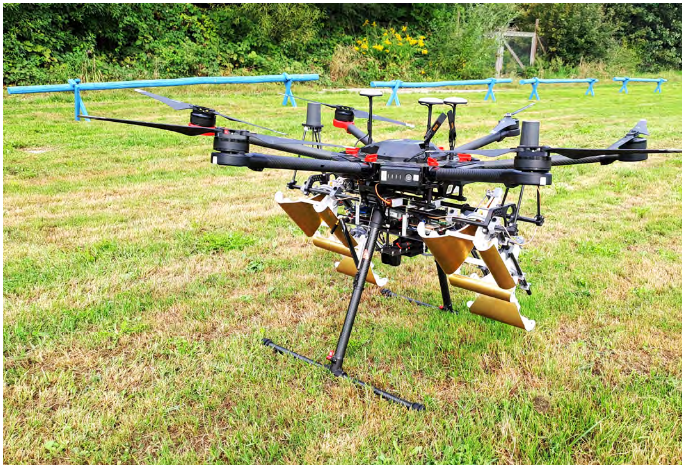
Uncrewed aerial vehicle (UAV) - based remote sensing capacities have progressed significantly in recent years, but further testing and evaluation is needed for them to prove impactful. UAV equipped with Ground Penetrating/Synthetic Aperture Radar (GP/SAR) in test field, Ulm, Germany. © GICHD 2025
