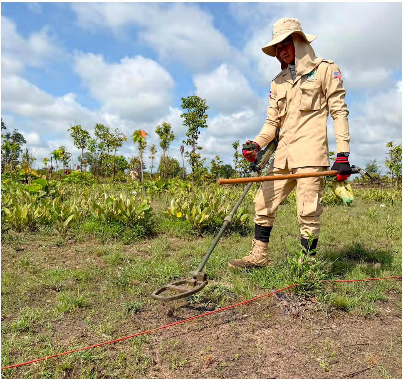
Metal detectors remain the most commonly used detection tool. Norwegian People's Aid (NPA) deminer using a handheld metal detector in a cluster munition remnants survey (CMRS) task in Ratanakiri, Cambodia. © GICHD 2026
