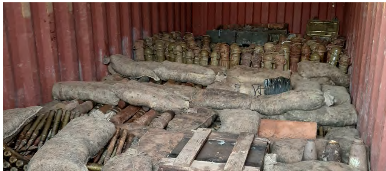
Poor ammunition storage in a shipping container
