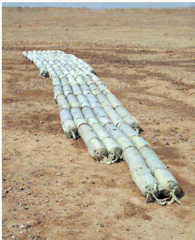
Figure 14 – Preparation of Propelling Charges for Open Burning. 80)
