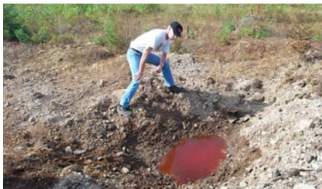
Figure 1: Standing water contaminated with 2,4,6- trinitrotoluene (TNT) and TNT light-catalysed degradation products with the tell-tale pink tint. TNT and associated degradation products have a degree of toxicity, and in certain circumstances present a risk to humans, animals and plants. Image ©igem.org
