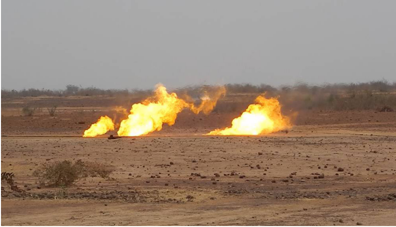
Figure 2: An open burn of old Soviet gun propellant in an arid environment, March 2016. Image© Swiss EOD Centre
