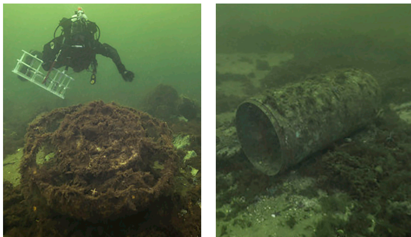
Figure 5: (left) a significantly corroded naval mine found at the munitions dump site in Kolberger Heide, at the entrance to Kiel Fjord in Germany; (right) a mine with no evidence of corrosion found in the same location. This demonstrates how varied the condition of ordnance can be even in very limited geographical environments and highlights how difficult it can be to predict environmental impact. Image© Jana Ulrich, FTZ Uni Kiel
