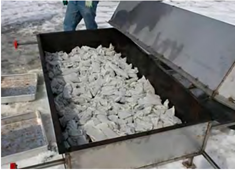
Figure 3: Prototype of the burn tray developed by Canada and the US, a) loaded with propellant prior to burn, and b) during disposal. The trays surrounding it were put in place to capture the mass of propellant deposited outside of the tray ( Images ©Dr Michael Walsh )
