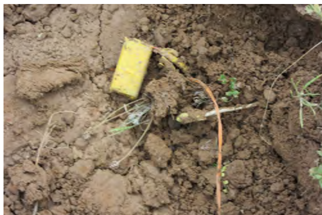
Figure 4. 9V battery used to power improvised landmine pressure plate switch (image credit: FSD).
