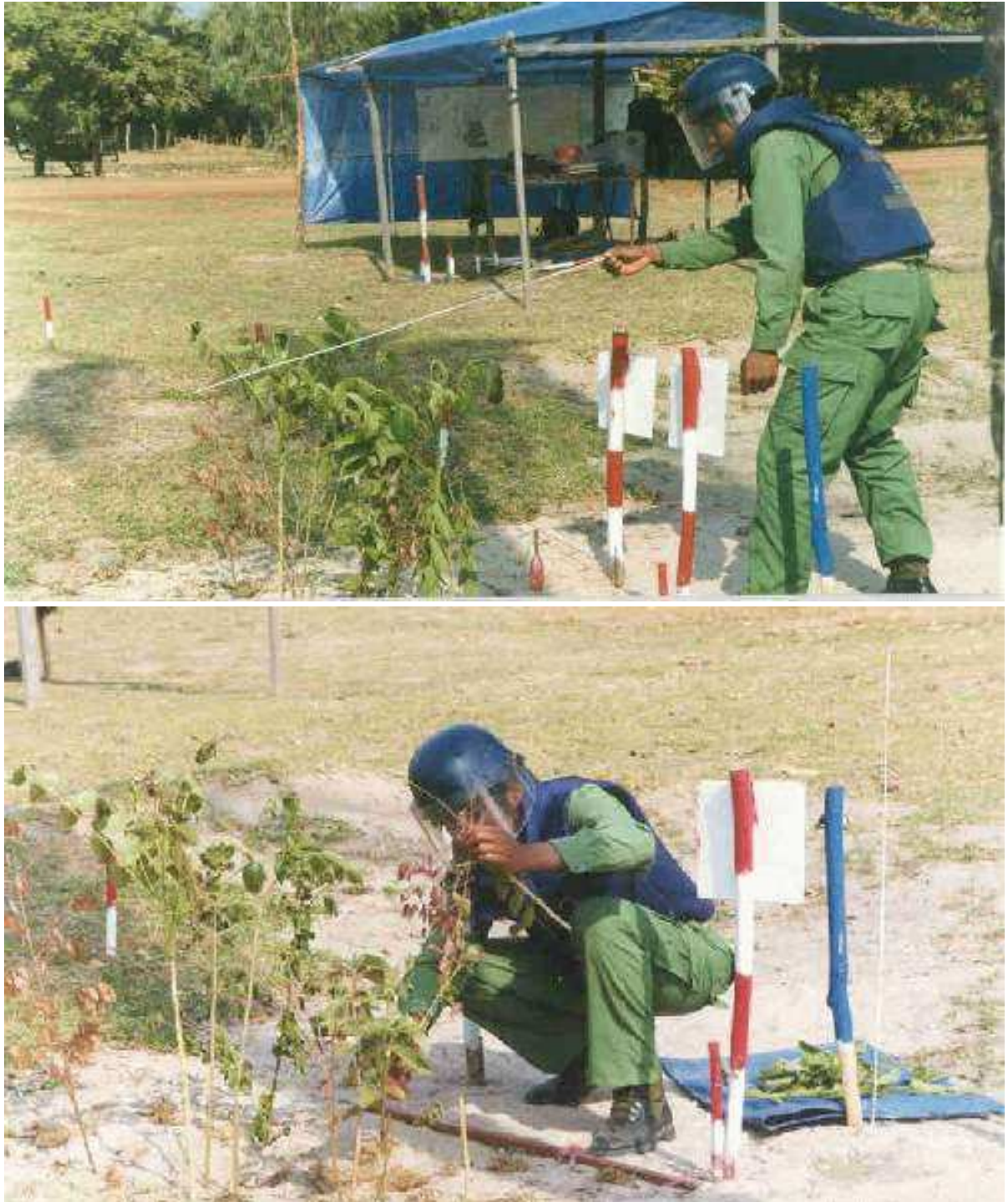
Figure 2.5: Sequence of operations, manual demining in Cambodia (part 1). — deminers demonstrating SOPs in a prepared safe area. Above: Tripwire detection using a bamboo wand Below: Vegetation cutting and removal.
