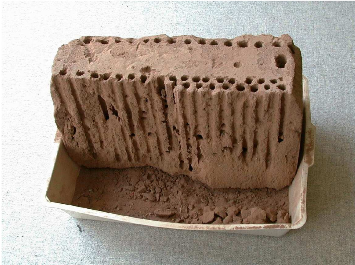
Figure 5.19: Block of “Soil A” sectioned to show clean parallel holes produced by rotary prodder.
