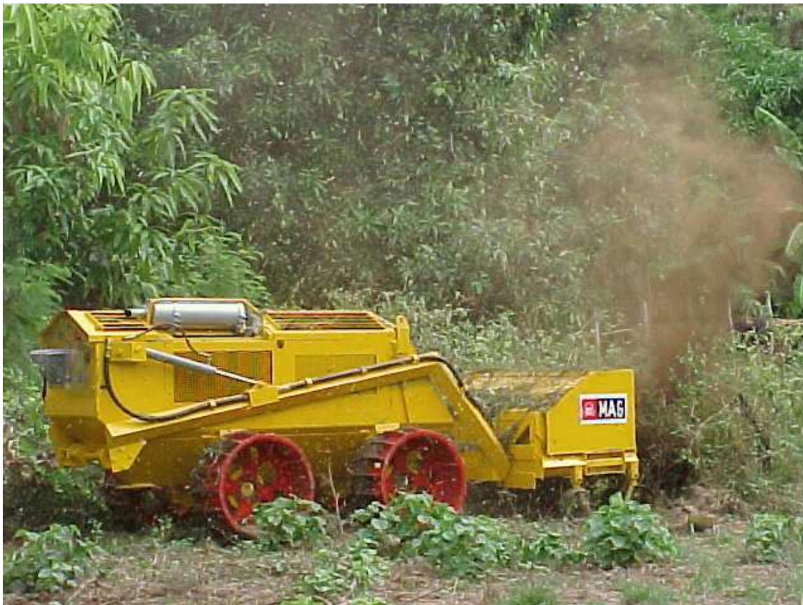
Figure 2.4: Tempest remote-control mini-flail with custom built blast resistant hull.
