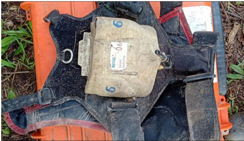
Figure 15 – SMART harness after a working day in the rainy season
