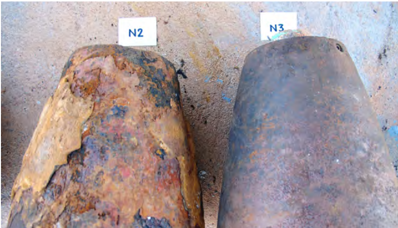
Nose sections of United States Mk 82 bombs dropped during the Indochina Wars and recovered, unexploded, in the early 2000s. These heavy steel casings were virtually unaffected by impact, other than the loss of paint coatings. Both have been exposed to water for nearly 50 years, but have corroded differently, possibly because of the soil conditions in which they were buried. The nose fuzes were heavily damaged on impact, but even the heaviest corrosion would still take several more decades to penetrate the steel casing. Image: Fenix Insight Ltd.
