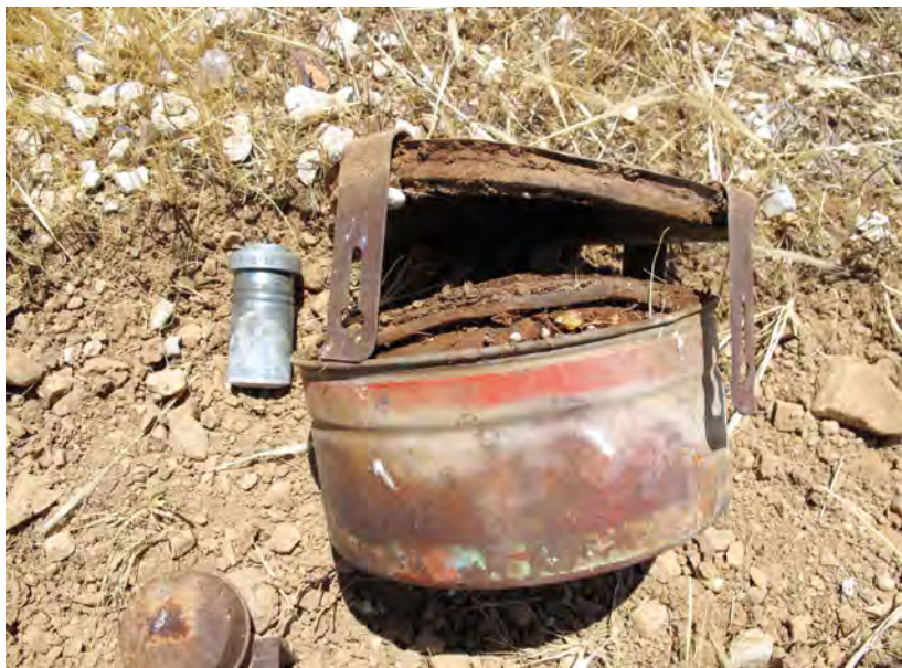
A British Mk 5 anti-tank mine in Jordan, with TNT being forced out of the casing by internal corrosion. This is an extremely rare instance where the fuze (to the left of the mine) may still be viable, but the loose structure of the main charge may be unable to sustain detonation. Usually, by this stage the fuze would have suffered numerous points of failure due to ageing. Image: Fenix Insight Ltd.
