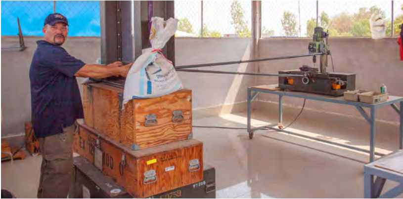
A Mechanical Remote Fuze Disassembly Kit (MRFDK) used for removing small energetic components such as primers in fuze rotors, Golden West Humanitarian Foundation GWHF Cambodia 2014. Specialist explosive processing facilities, whether permanent or mobile, may be needed to fully ascertain the effects of ageing on explosive ordnance. Image: GICHD.
