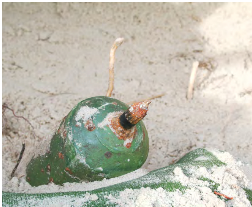
A stockmine with ZZ-42 igniter found buried in the sand dunes at Skallingen, September 2006. While the mine body, consisting of metal fragmentation embedded in concrete, has proved very resilient, with the paint still showing, and the bakelite fuze body is intact, the exposed part of the striker has heavily corroded. The fuze is no longer functional, although it could still pose an explosive hazard.
