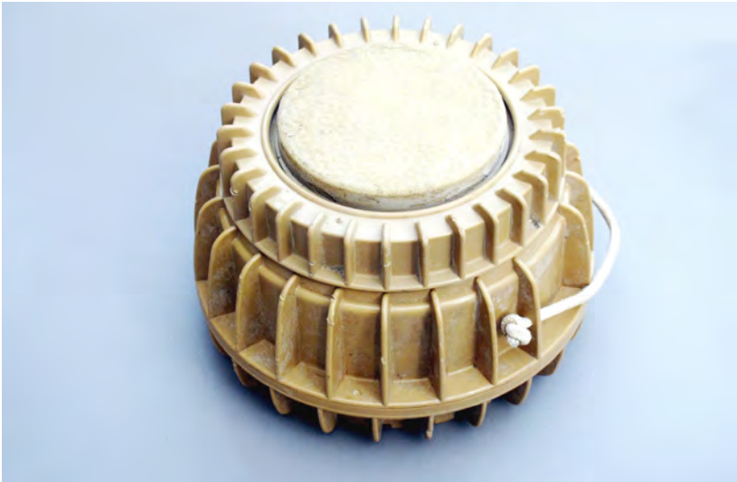
The Italian TC/6 anti-tank mine is one of many designs that use a pneumatic transfer system. When mines are exposed to heat or sunlight for prolonged periods, the elastomer pressure plate becomes brittle, causing the seal around the shoulder to fail. Once air is allowed to escape from beneath the pressure plate, the pneumatic actuation system can no longer operate. Image: Fenix Insight Ltd.
