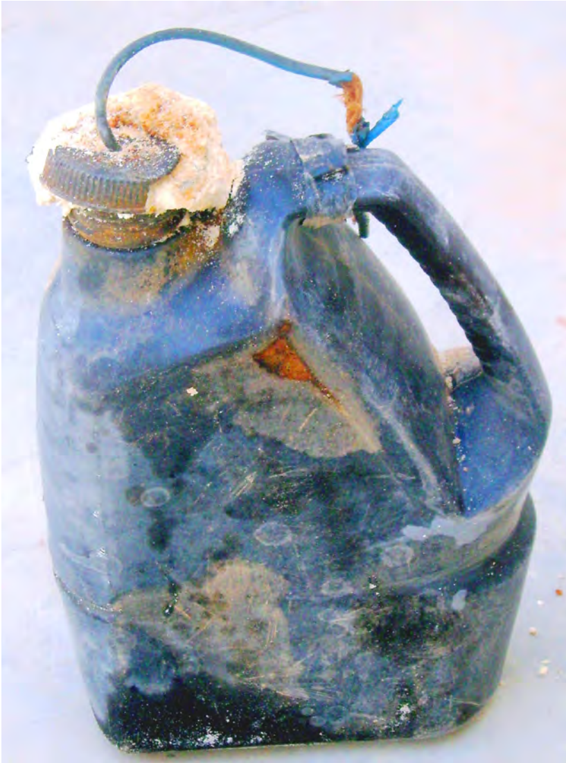
Ammonium Nitrate exudation from the neck of a 5ltr Improvised Plastic IED, Khan Village, Kobane, Syria, July 2016. This main charge was probably emplaced at some point in 2014. It is likely a result of phase changes due to temperature causing expansion and rupturing of the casing at the screw thread. The booster charge was fashioned from knotted detonation cord, which is also prone to hydroscopic action if water breaches the casing. Image: Bob Gravett.
