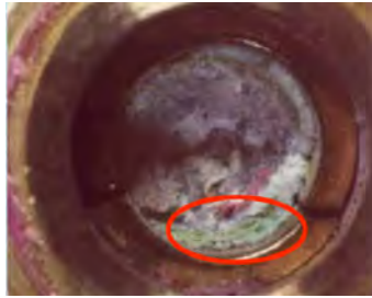
A photo from the Dutch Safety Board accident investigation showing green copper azide crystals (circled) inside the casing of an M-6 mortar bomb fuze. The formation of this sensitive compound is believed to have caused a fatal accident in 2017, and could become a hazard in many types of ammunition as it ages. Image: The Netherlands Organisation for Applied Scientific Research.
