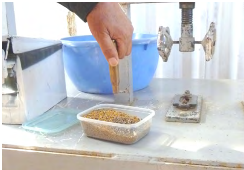
Double based propellant removed from debulleted 12.7 x 107mm ammunition. The propellant contains stabilizers to absorb the nitrogen oxides emitted by the degradation of nitrocellulose. Such stabilizers are used up over time and ammunition containing propellant can become a fire hazard. This risk increases in hot environments. It is for this reason that AXO found in the field containing propellant should not normally be stored in an ASAs or explosive stores. Image: Roly Evans.
