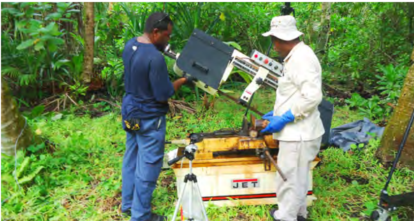
A portable cutting deck, based on a commercial bandsaw, conducting exploitation of Japanese 75mm Type 94 HE projectiles. While not a conventional ammunition process facility, mobile cutting stations can still conduct exploitation safely by effectively controlling the surrounding around as a range. All cuts are conducted remotely. The TNT fill is ultimately disposed of by open burning. Image: Len Austin.
