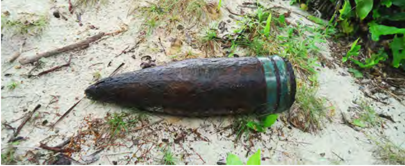
A Japanese 15 cm Type 13 or 88 Common projectile, showing deep corrosion from exposure to seawater. The copper driving bands are now green due to the copper salts produced by chemical reaction with the local environment. The smooth driving bands indicate that this projectile has never been fired. This classifies it as abandoned (AXO) rather than unexploded (UXO) explosive ordnance. While its fuze may be considered not armed, AXO still poses a significant explosive hazard. It can be misused by fishermen. In other countries AXO has frequently been employed as a main charge in IEDs. Image: Len Austin.
