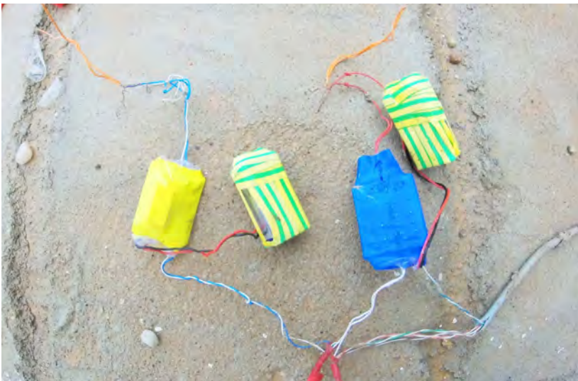
9v batteries recovered from victim operated IEDs, Iraq, December 2016. How long a 9v battery retains its potential is a key consideration in how long the device remains viable. Image: Bob Gravett.
