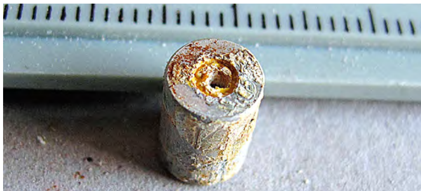
A detonator assembly from an Italian SB-33 mine, laid in the Falkland Islands/Malvinas in 1982 and recovered 35 years later. The hole in the top shows that, at some point, the mine had been actuated and the mechanical components of the fuze mechanism have functioned correctly, driving the firing pin into the stab receptor. But the detonator failed to function and the mine remained unexploded. It is probable that prolonged saturation or damp has caused this failure. Image: Fenix Insight Ltd.
