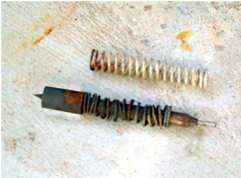
The striker and spring from a Russian PMN mine recovered in Cambodia, 2014, with an example of the spring in good condition, above. The corroded spring has lost its ability to drive the striker into the detonator assembly; in other words, it can no longer supply the energy needed to allow the initiation sequence to reach the next stage. This will prevent the mine from functioning as designed and is typical of many such applications within fuzes. Image: Fenix Insight Ltd.
