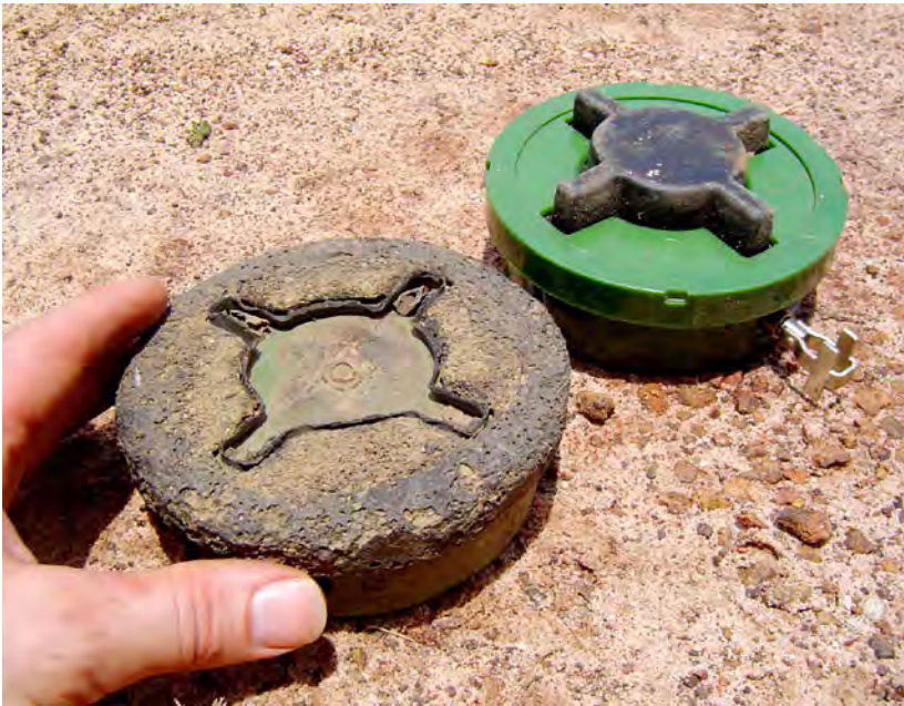
Russian PMN-2 anti-personnel mines recovered from different minefields in northern Cambodia in 2009. The mine in the foreground has been severely damaged by fire, which has burned away the cruciform pressure plate and allowed water to enter the mine. The explosive components are undamaged but, ironically, the loss of the pressure plate means that this mine could no longer function as designed.
