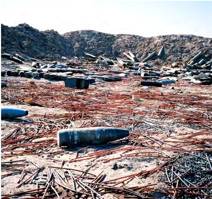
An ammunition depot in Iraq, 2003. Looters seeking brass cartridge cases have tipped unwanted double-based propellant out onto the ground, where it becomes dry and brittle in the hot sun. In this state, propellant is highly vulnerable to ignition by heat and friction. Image: Fenix Insight Ltd.
