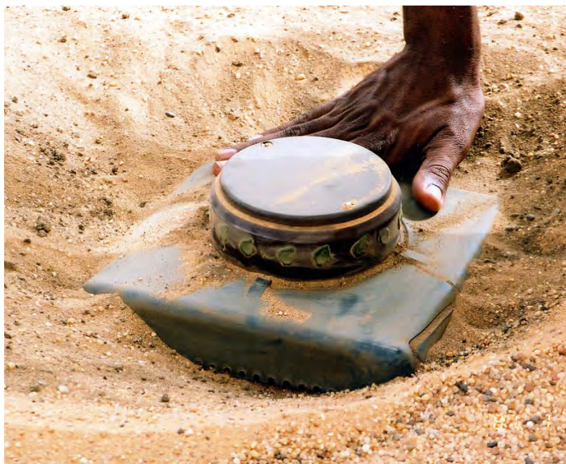
A PRB M3 mine in northern Chad. The mine was buried and had thus been largely protected from UV light. In this instance the high temperature has caused a split in the polythene mine casing. The bakelite fuze assembly has on the other hand remained intact. Different plastic materials age at different rates even in the same conditions. Bakelite is a remarkably resilient material that is even difficult to penetrate with thermite torches. Image: Fenix Insight Ltd.
