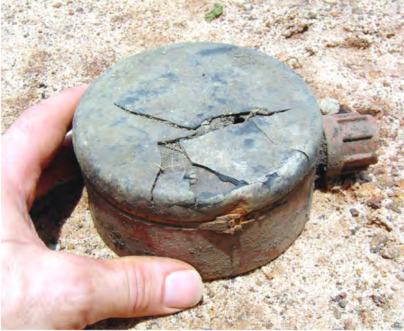
A Russian PMN anti-personnel mine recovered in Afghanistan in 2010. This mine was left on the surface and suffered prolonged exposure to sunlight. The rubber has lost its flexibility and become extremely brittle, resulting in the formation of cracks and loss of some sections. This has breached the integrity of the casing and allowed water to enter the mine, causing corrosion damage to the internal mechanical mechanism, particularly the spring that supports the last holding device in the mine but also the coiled spring that is part of the striker assembly. The bakelite body of the mine is remarkably resilient however. Image: Fenix Insight Ltd.
