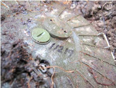
While the mine's glass reinforced polycarbonate casing is extremely resilient, the mine's detonator plug was not properly tightened when the mine was laid.
