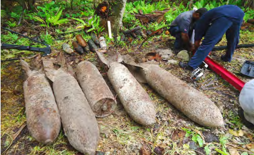
Recovery of Japanese bombs from a buried stockpile. These Type 3 No25 Mk8 Mod1 – 7 bombs are unfuzed, with just a blanking plug fitted into the fuze wells. The absence of a fuze and primary explosive reduces the risk significantly. While a degree of corrosion can be seen, the resilience of the thick cased munitions is evident. Image: Len Austin.
