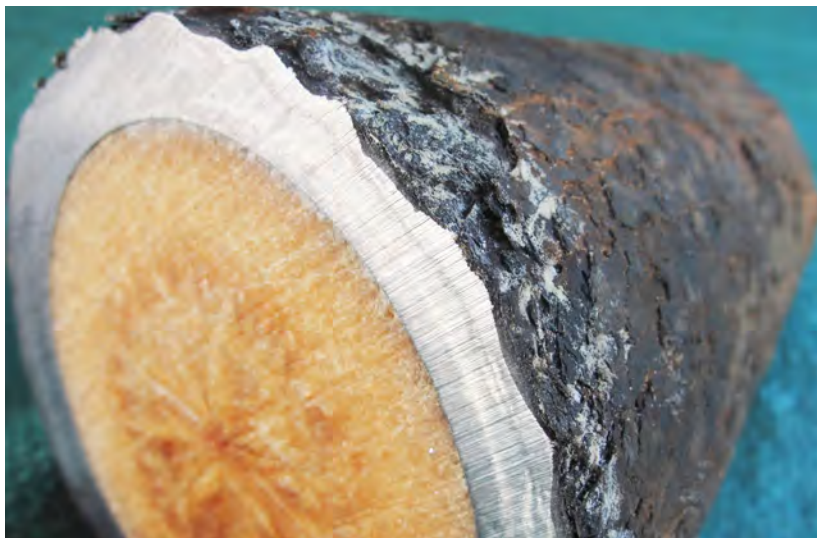
The casing of an unexploded M107 projectile, recovered around 50 years after it was used in Vietnam. A section through the projectile shows the surface is heavily corroded, although the steel beneath is in remarkably good condition. Under some circumstances, a superficial iron oxide rust layer may provide protection that slows down the corrosion process. Image: Fenix Insight Ltd.
