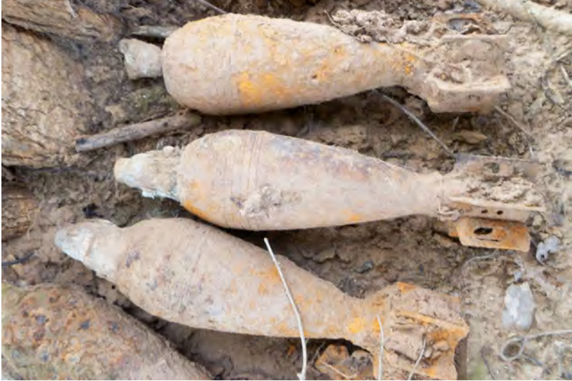
Weathered AXO gathered by local farmers. Note that corrosion of the fuze is more advanced than on the mortar bodies. Image: Roly Evans.
