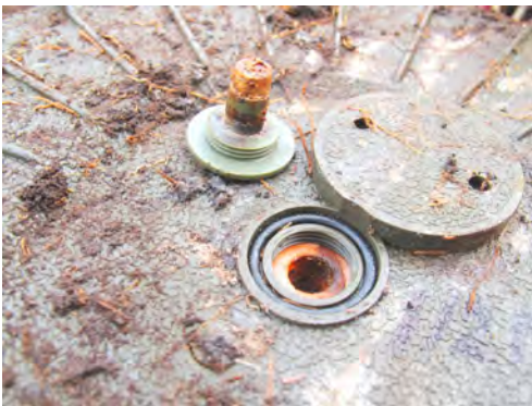
Examination shows that the loose plug allowed water to enter the casing, saturating the detonator over time.
