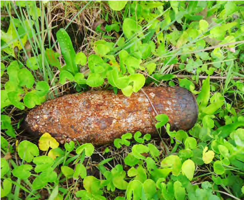
A fired Japanese Type 91 15.5 cm HE projectile, showing heavy external corrosion.
